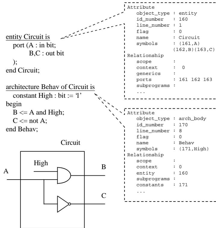
Figure 4. Data structure of VDT object.
