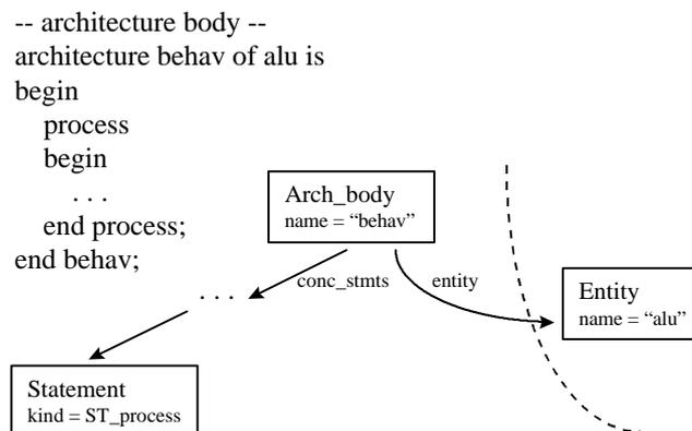
Figure 7. Intermediate form representation for architecture body.
