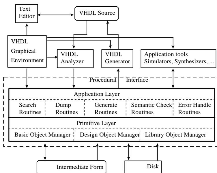
Figure 1. Structure of VHDL Developer's Toolkit
