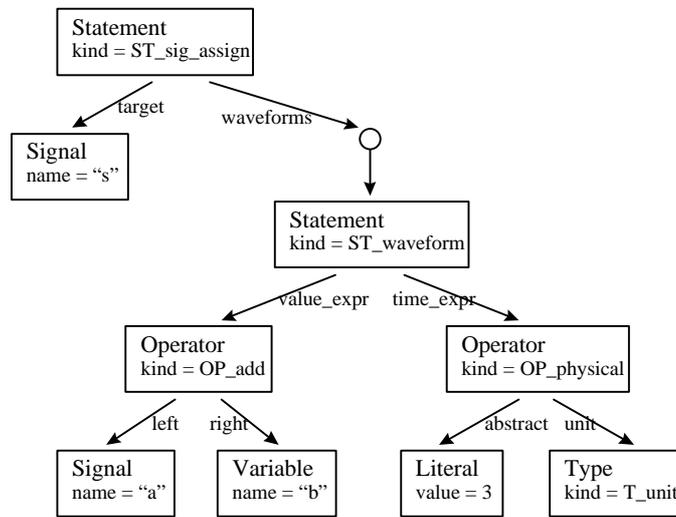
Figure 9. Intermediate form representation of signal assignment statement.
